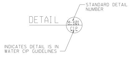
A CITY OF SAN DIEGO STANDARD DETAIL IS CALLED OUT ON PLAN OR SECTION AS:
