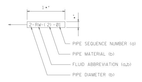
(a) THIS ELEMENT WILL BE SHOWN ON P&ID (b) THIS ELEMENT WILL BE SHOWN ON YARD PIPING AND MECHANICAL DETAILS
