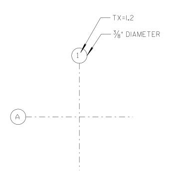
USE A CENTERLINE AS A COLUMN LINE. EXTEND THE LINE 1/4" BEYOND THE VIEW AT BOTH ENDS, AND TERMINATE IT AT THE TOP OR THE LEFT SIDE WITH A COLUMN LINE BALLON.
